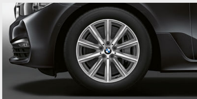
□ 18" light alloy wheels V-spoke style 684 Ferric Grey gloss-lathed, 8J x 18 with 245/50 R18 tyres.
